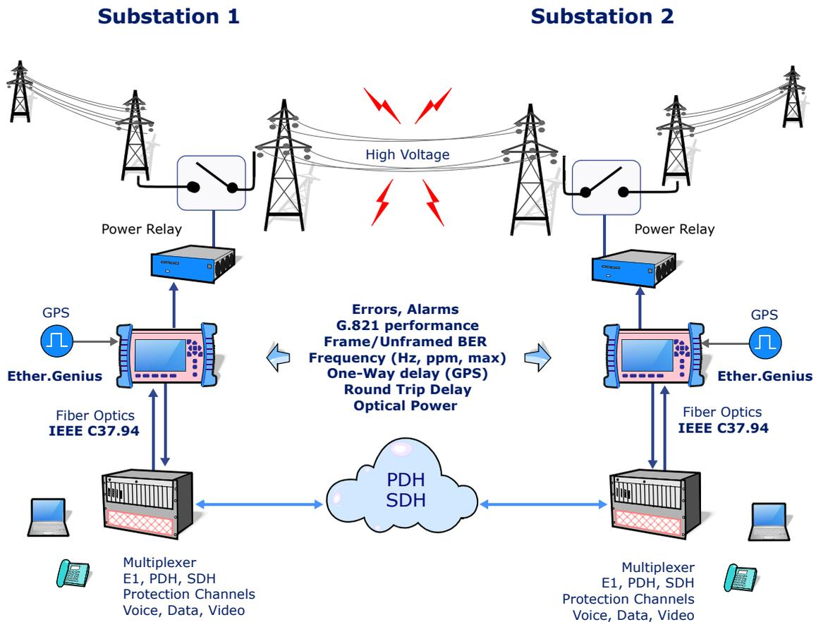
Figure 4 Teleprotection system installation and maintenance with ALBEDO Ether.Genius.
