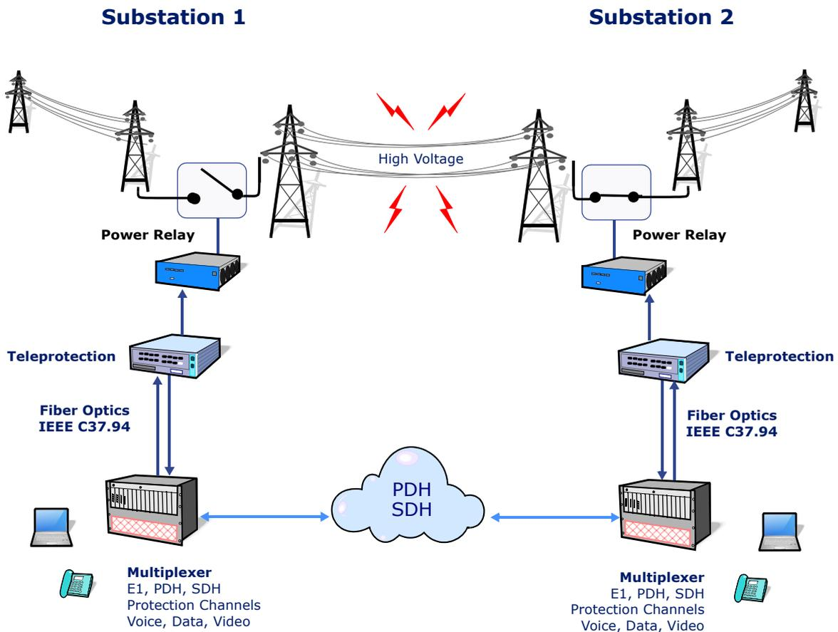
Figure 2 Teleprotection architecture using C37.94 in normal operation.
