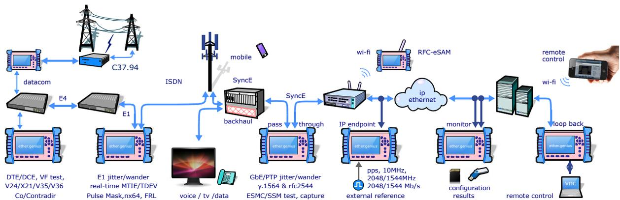
**Figure 3** *Ether.Genius* is a multi technology tester equipped with all the features to install and troubleshoot C37.94 teleprotection systems and Gigabit Ethernet, SyncE, PTP, E1 and Datacom services.
